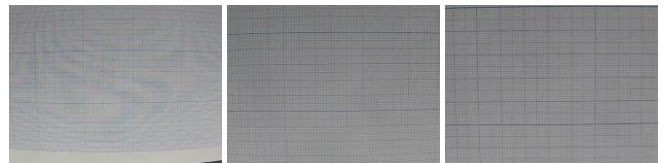
Fig. 4. Image acquired with GoPro at 1280 x 720 resolution, 14mm focal length (left image, pronounced barrel distortion), 21 mm focal length (central image, significant barrel distortion) and 28 mm focal length (right image, slight barrel distortion).
