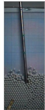
Fig.10. b) The test object path is reoriented by the border between the two regions. A gap between the two regions it formed, and it favors a deeper penetration of the test object.
