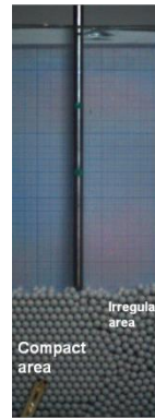
Fig.10. a) On the left side of the image, the particles are arranged and forms a compact region; on the right side, their placement is irregular. The test object impacts the plastic particles right on the separation zone between the two region.
