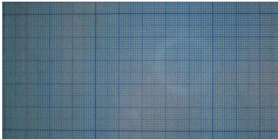
Fig. 2. Image acquired with Fastec camera and Navitar lens. There is no geometric distortion in the image
